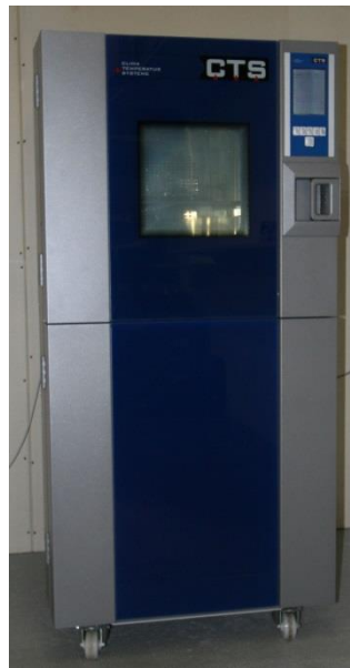
Figure 5: Overall view of the temperature test chamber
